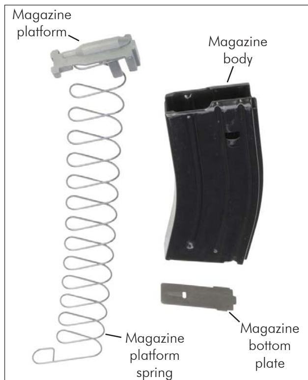
Fig. 7.2.b - Disassembly of the magazine (601)
