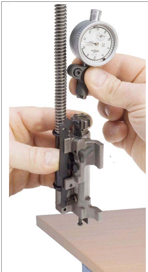
Fig. 10.5.d - Positioning of the firing pin protrusion gauge G121
