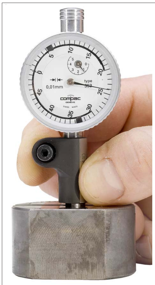
Fig. 10.5.b - Fit the firing pin protrusion gauge G121) into the reference gauge for zeroing G122
