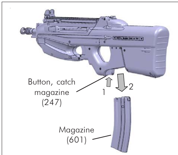
Fig. 4.2.b - Removal of the magazine (601)
