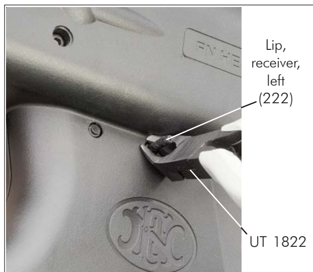
Fig. 9.3.ah - Cutting the lugs of the lip, receiver, left (222)
