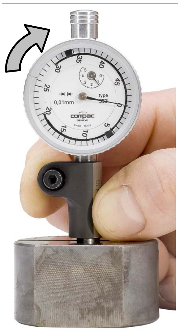
Fig. 10.5.c - Reset the firing pin protrusion gauge G121
